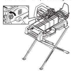
· Hold down the button for locking the blade shaft.
