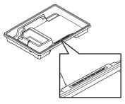
Slide out the slurry collector tray and flip up the slurry collector tray extension.
