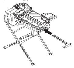
• Connect the water hose (2) and the water pump (1) to the connectors on the frame.
