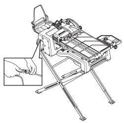
Make sure the water level is maintained at this level when cutting.
