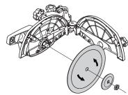
· Close the blade guard. Tighten the locking knob.
