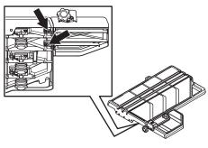
Screw the cutting guide onto the conveyor cart. The guide can be folded outwards for angled cuts. Use the angle markings on the cutting guide to set the correct angle.
