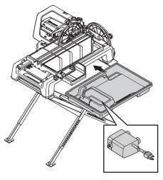
• Fill the water tray with water up to the marked level.
