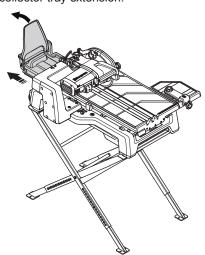
With a push, the slurry collector tray can be locked in its inner position.
